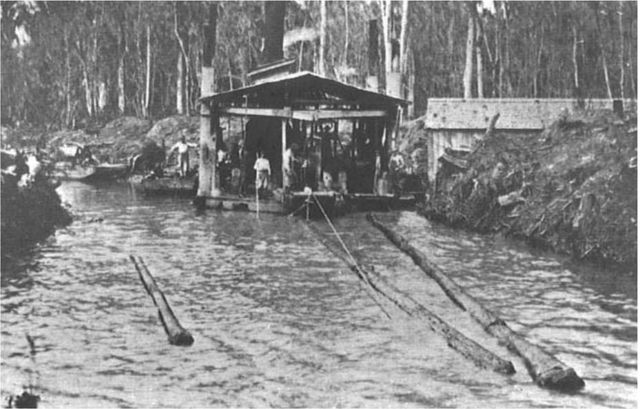
*Figure 4-3. In the late 1800s, William Baptist of New Orleans developed the pullboat system for logging cypress. This two-drum pullboat could skid logs for up to 3,000 feet from the swamp (from Williams, M. 1989. *The lumberman's assault on the southern forest, 1880-1920*. p. 238-288 in M. Williams (ed.) *Americans and Their Forests: A Historical Geography*. Cambridge University Press, Cambridge, UK).*
